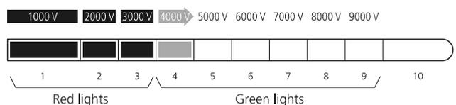
If you see only red lights at each pulse and no green lights, this means that your fence line is very heavily loaded, and you need to look for faults on the fence line. See *Using the fault finder* on page 3.
