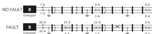
If voltage has dropped on the fence system, it is necessary to identify the cause. (See *Frequently asked questions/Troubleshooting* on page 8.) Possible causes of poor fence performance are short circuits or arcing faults. Location and repair of these faults is often difficult. The fault finding function has been developed to reduce the amount of time spent in locating fence line faults. Regular use of the fault finder will increase your familiarity with the fence system.
